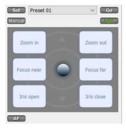
With a Pan-Tilt-Zoom (PTZ) camera, an operator can manipulate the camera's direction, Zoom, focal distance (Focus), and amount of light (Iris). The operator can also control pre-configured camera views called "Presets".
